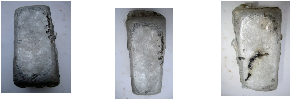
Figure 4: Actual Shrinkage for 40mm, 50mm and 60mm of Rectangular Objects Without Feeder
